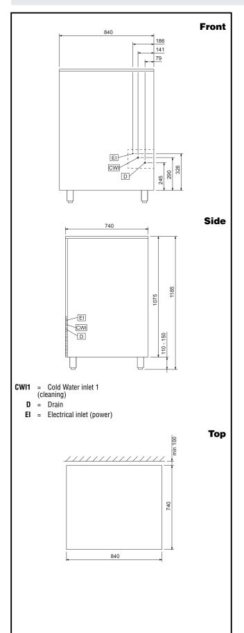
**Electric** Supply voltage: 730531 (FGC120A) 220-240 V/1N ph/50 Hz Electrical power max.: 1.05 kW **Capacity:** Bin capacity: 65 kg **Key Information: External dimensions, Width:** 840 mm **External dimensions, Depth:** 740 mm **External dimensions, Height:** 1185 mm Net weight: 113 kg Output: 130 kg/day Kind of cube: Ice Cube 18 g **Sustainability**
